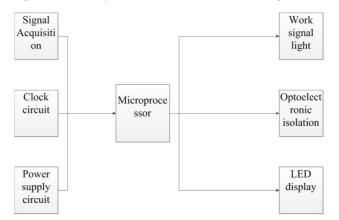
Fig. 2. Composition of intelligent control system
